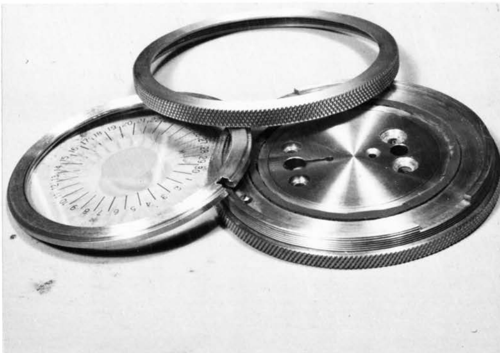
Figure 8. - Graduated glass disk and rotating ring with base plate
