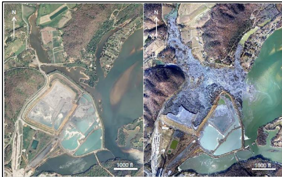
Figure 5.12: Aerial images before and after the landfill failure in Tennessee, 2008 (Source: http://www.cnn.com/2009/HEALTH/07/13/coal.ash.illnesses/index.html?eref=rssus ).
