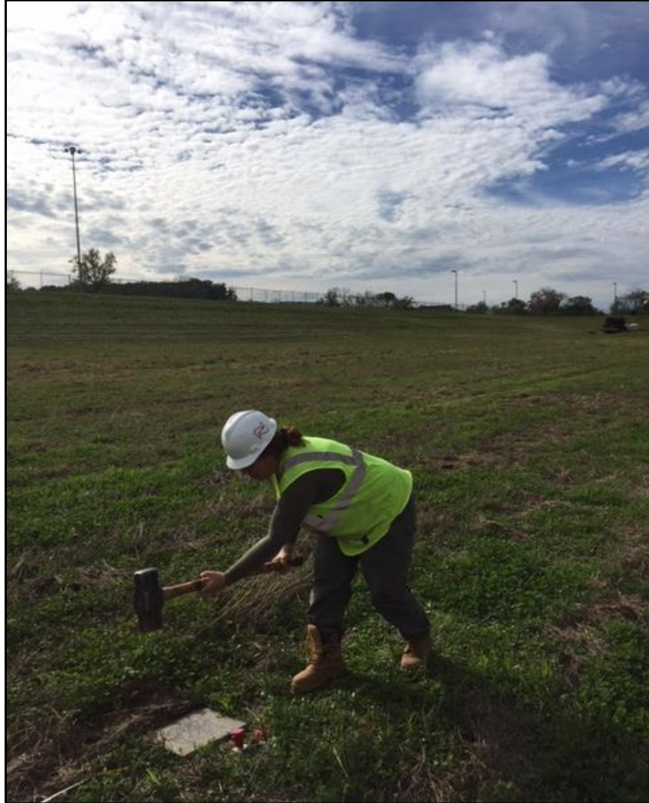
Figure 7.4: Acquisition of MASW data in the field.
