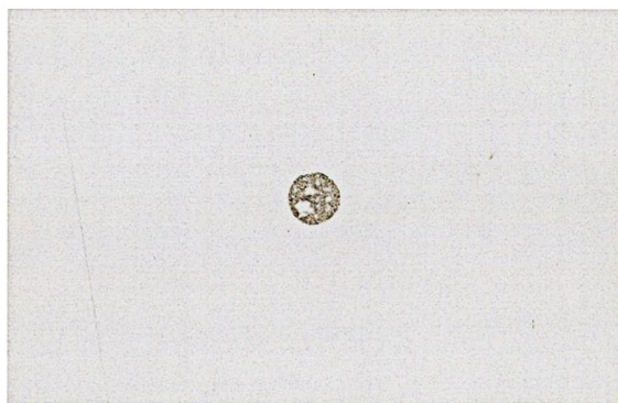
Fig. 31 - Specimen W-80; sulphur print; transverse section.
