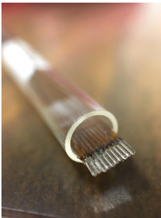
Figure 1. Photograph of a 10-capillary Gradient CapPack contained in a 5-mm NMR sample tube.
