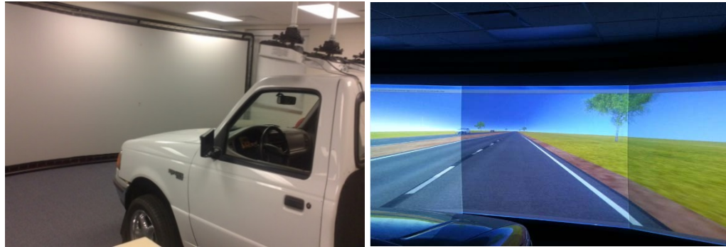
Figure 2. Driving simulator (left) and the screen view (right)
