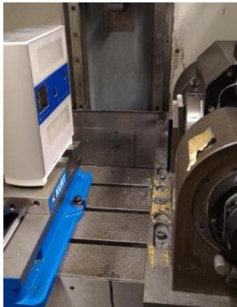
Figure 14. Scanning the part before machining
