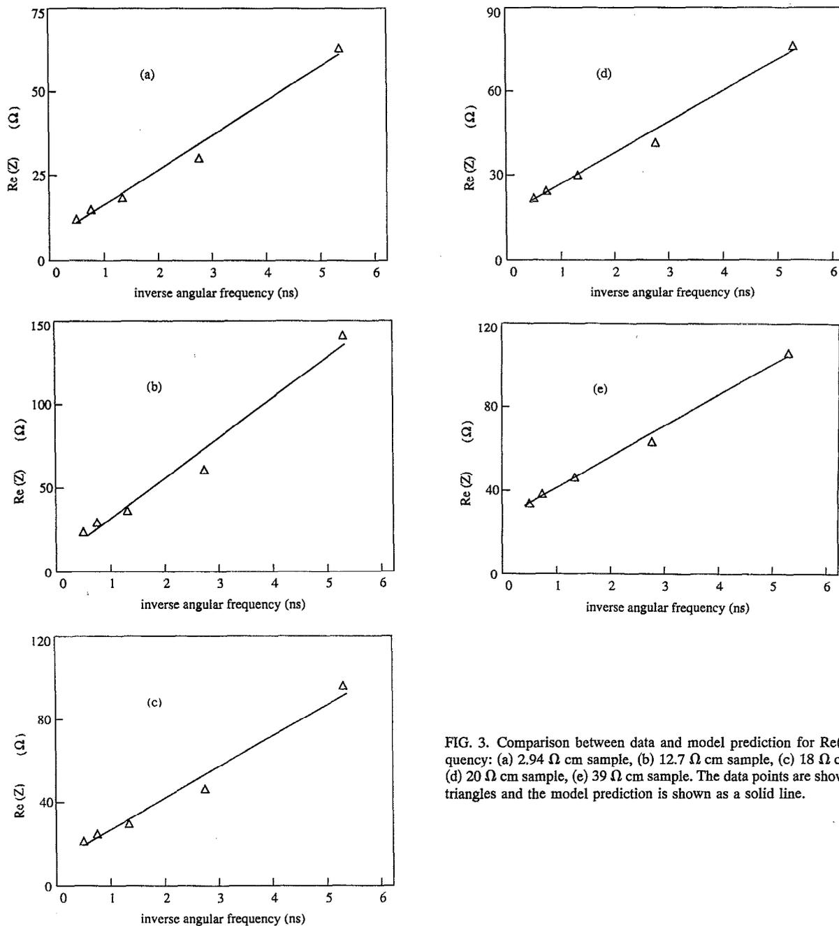
FIG. 3. Comparison between data and model prediction for  $Re(Z)$  vs frequency: (a) 2.94  $\Omega$  cm sample, (b) 12.7  $\Omega$  cm sample, (c) 18  $\Omega$  cm sample, (d) 20  $\Omega$  cm sample, (e) 39  $\Omega$  cm sample. The data points are shown as open triangles and the model prediction is shown as a solid line.
