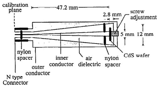
FIG. 1. Conical-coaxial test fixture detail.
