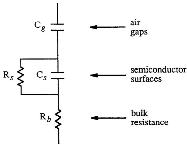
FIG. 2. Wafer impedance circuit model.
