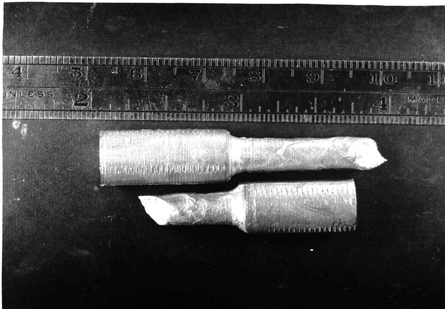
Figure 58. Cadmium-zinc-eutectic-alloy broken in tension.
