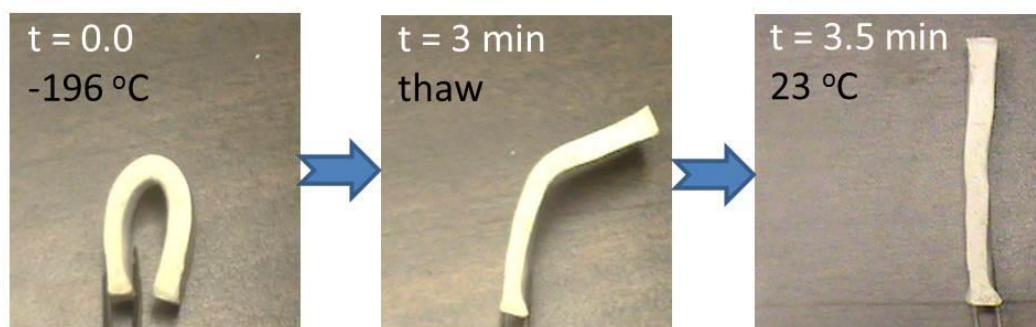
Figure 1.11. Shape memory aerogel demonstrating superelasticity at room temperature shape memory effect. (a). Sample was bent at RT allowed to recover. (b). Sample was first bent, then cooled to liquid N 2 temperature, and finally allowed to thaw at room temperature.
