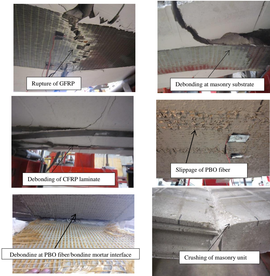
Figure 6. Typical mode of failures
