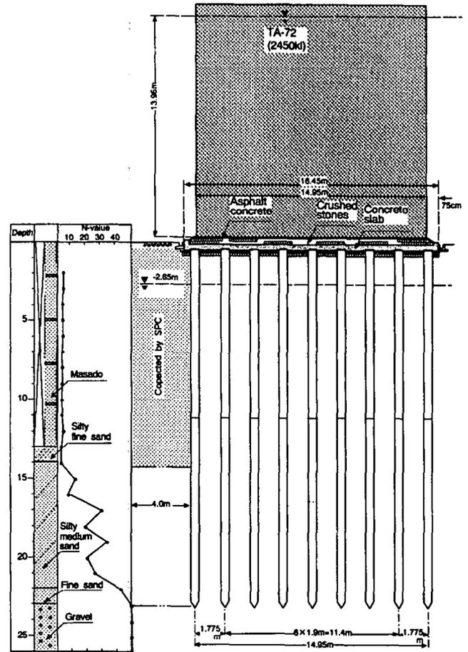
Fig. 2 Cross sectional view of tank TA72 and its foundation
