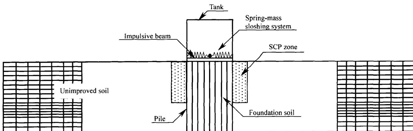
Fig. 7 Numerical model of the soil-pile-tank-fluid system
