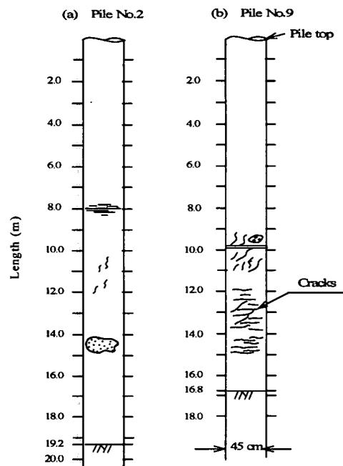
Fig. 5 Observed damage to piles of tank TA72: (a) Pile No. 2; (b) Pile No. 9
