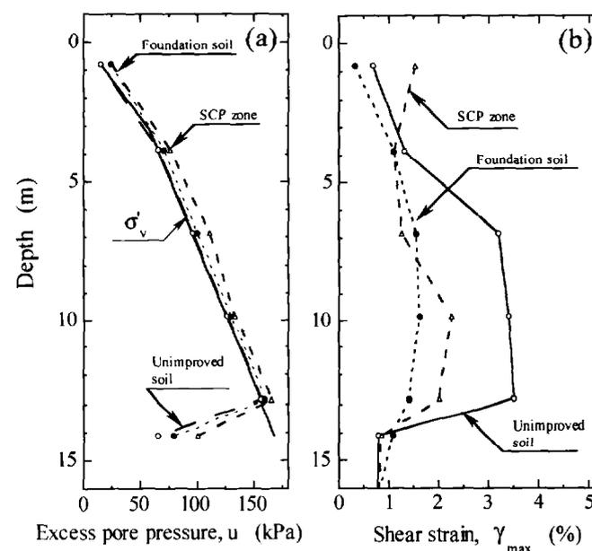
Fig. 8 Computed ground response: (a) maximum excess pore water pressures; (b) maximum shear strains
