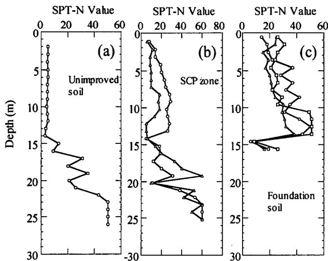
Fig. 4 SPT profiles: (a) unimproved soil; (b) SCP zone; (c) foundation soil
