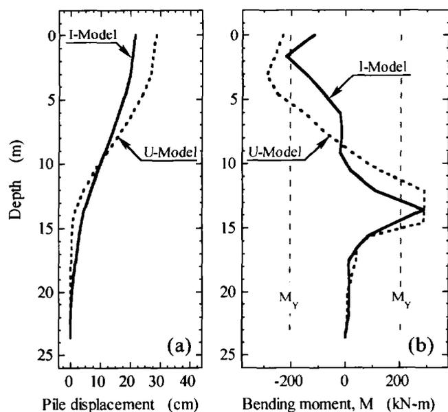
Fig. 9 Computed response of piles: (a) displacements; (b) bending moments
