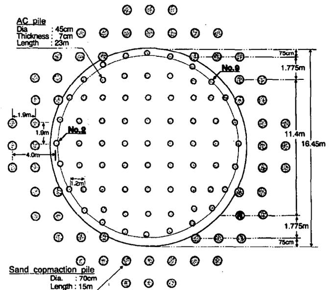
Fig. 3 Plan view of foundation
