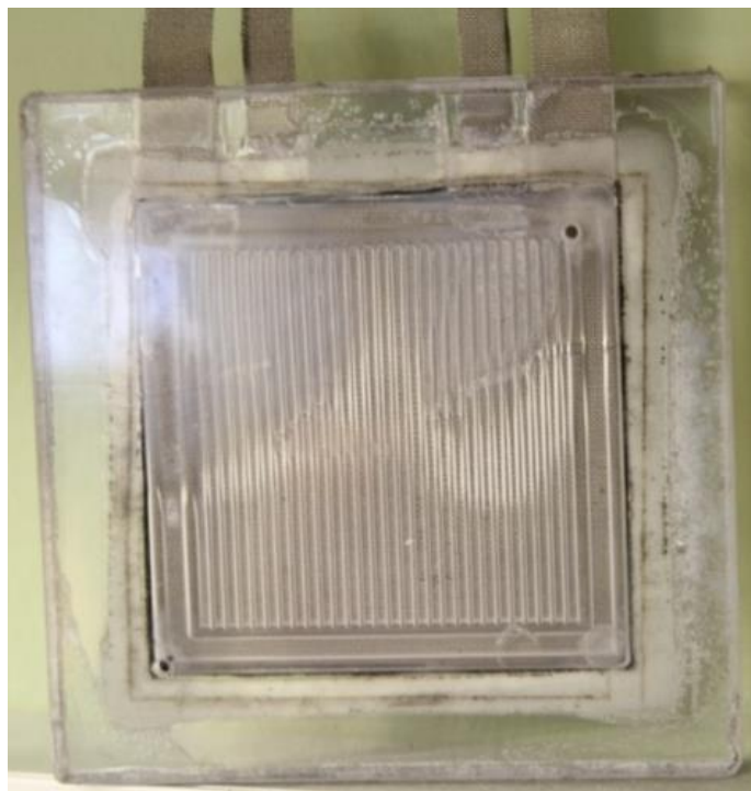
Figure 7: PEMFC prototype manufactured using the new design strategy
