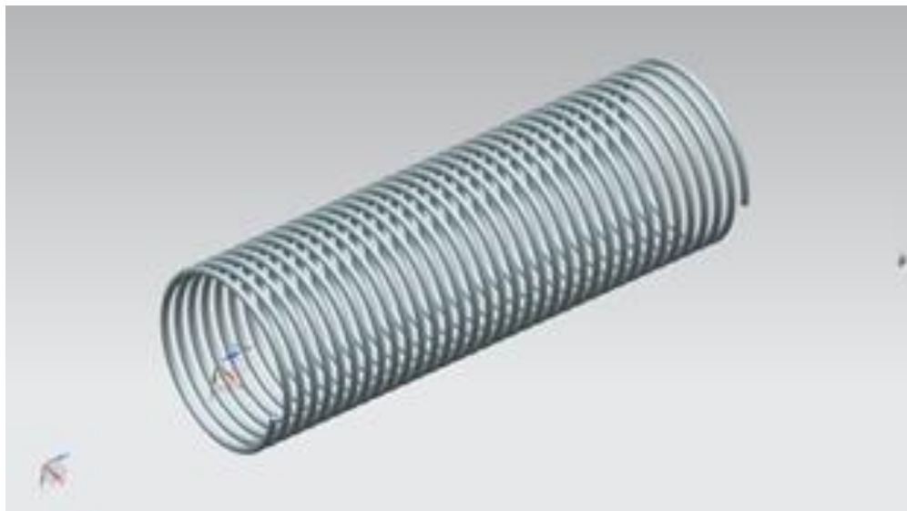
Figure 3: Helical flow sections with multiple 90° elbow bends
