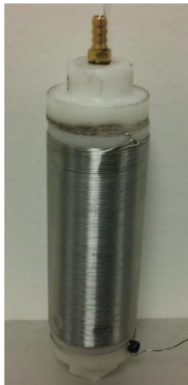
Figure 18: Prototype of chimney shaped air-breathing PEM fuel cell
