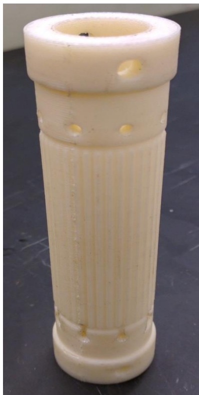
Figure 17: Chimney shaped mandrel manufactured using FDM
