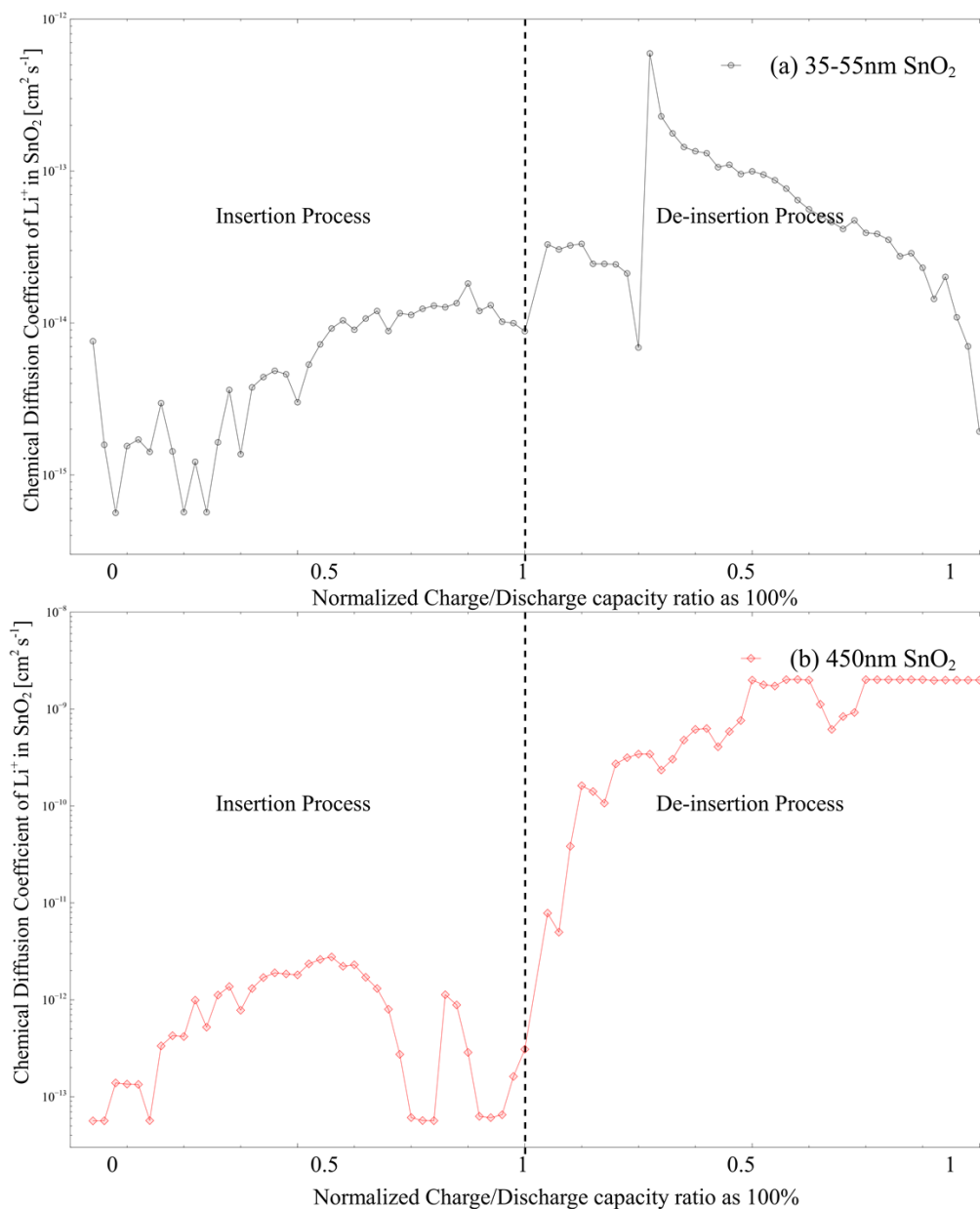
Figure 5.10. Calculated lithium diffusion coefficients for commercial \text{SnO}_2 nano particles with particle size of (a) 35-55, and (b) 450 nm. Left half of each panel shows lithium insertion process and right half shows lithium de-insertion process.
