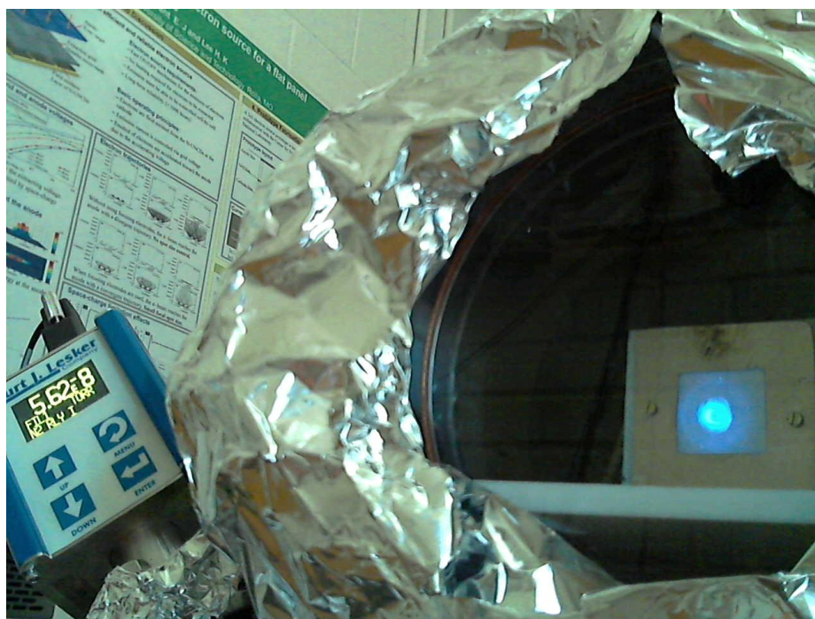
Figure 4.15. Electron beam visualization via YAG coated glass.
