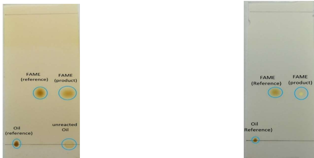
Figure 1.14: TLC separation of reaction mixture showing (a) incomplete reaction (b) completion of reaction
