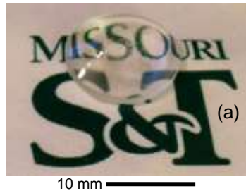
Figure 4.1 Convex shape made using filament-fed glass AM process
