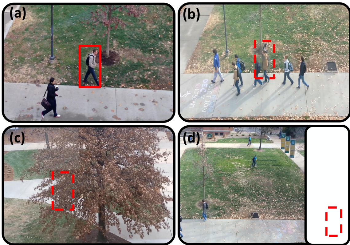
Figure 4.1. Visual people tracking and its challenges. (a) Successful tracking; (b) The target is occluded by other people; (c) The target is occluded by a tree over a long period; (d) The target moves out of the field of view temporarily.
