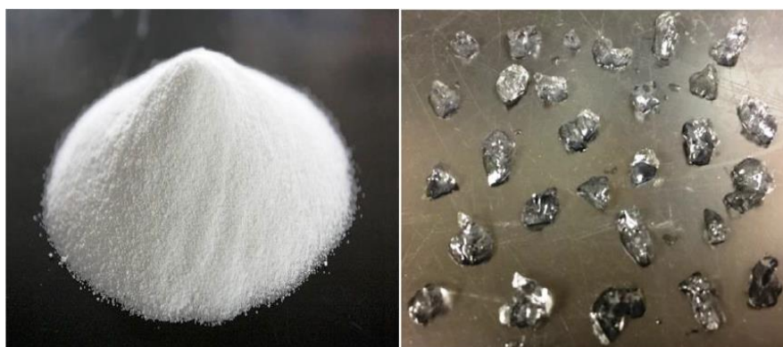
Figure 2.14. Dry and Swollen Preformed Gel Particles (Imqam et al. 2016)
