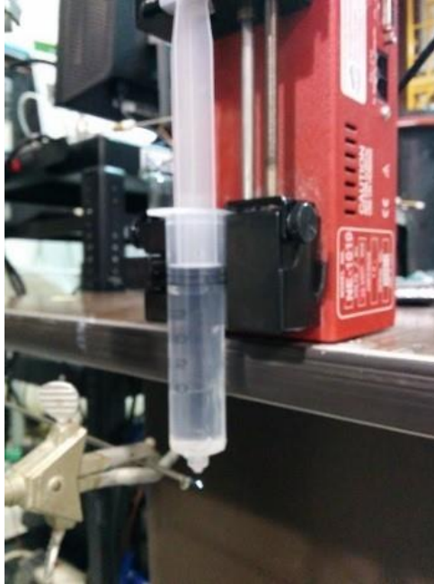
Figure 20. Syringe Pump with Two-Tip Optical Probe
