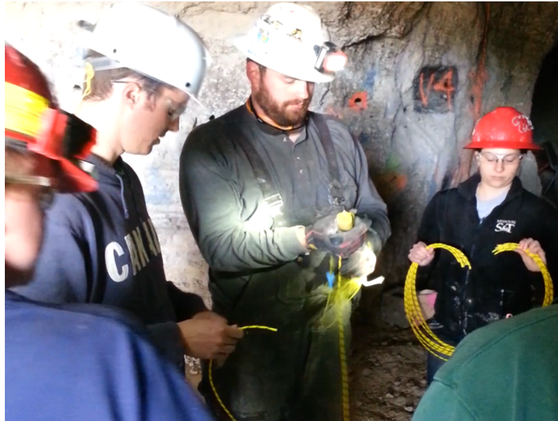
Figure A.2. Fixing a detonating cord to explosive material
