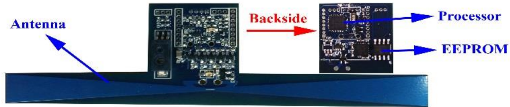
Figure 5.2. Modified WISP: Class-1 Generation-2 UHF passive RFID tag platform.
