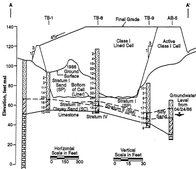
Figure 3. Typical soil profile along Section A-A'.
