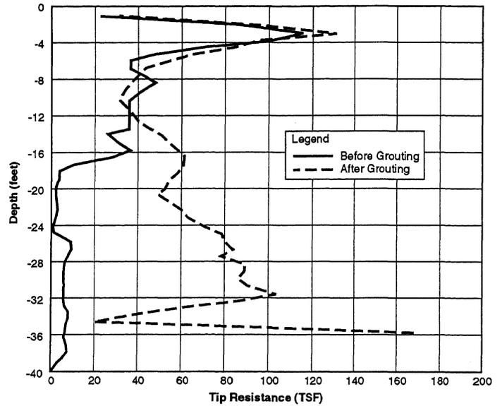
Figure 7. Comparison of tip resistances at CPT-4.
