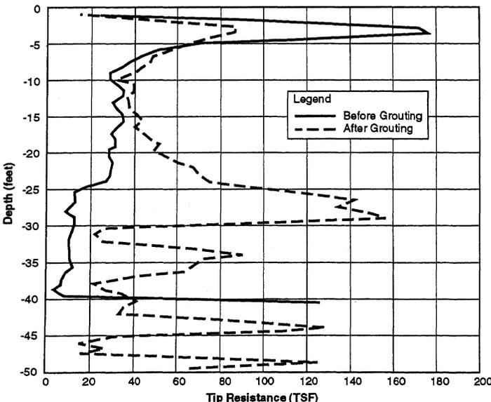
Figure 6. Comparison of tip resistances at CPT-3.
