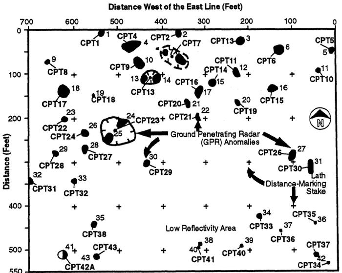
Figure 5. Potential anomalies and CPT sounding locations.
