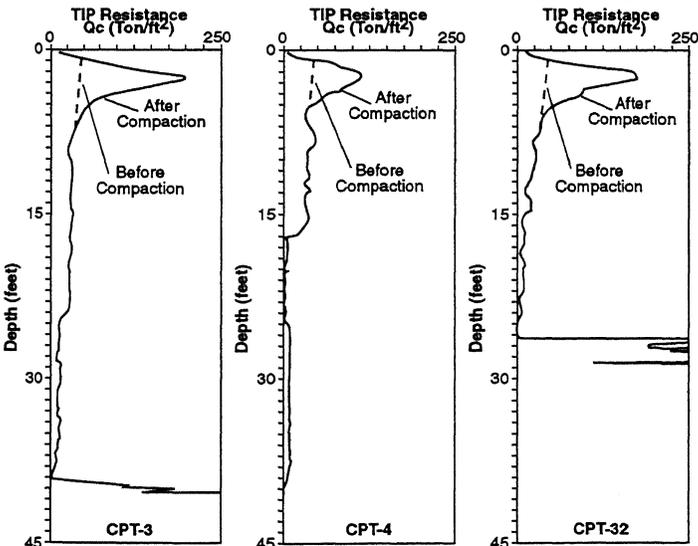
Figure 4. Sounding logs at CPT-3, -4, and -32.
