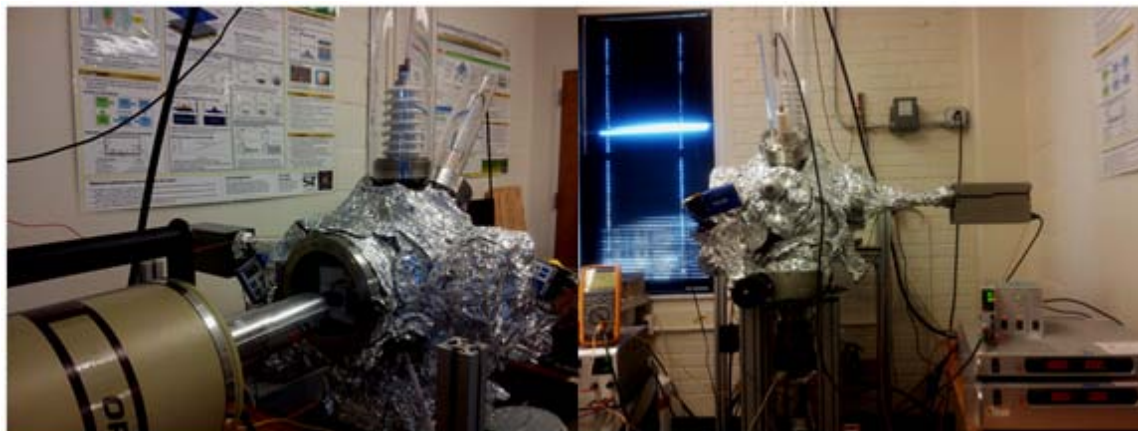
Figure 4.3. Experimental Apparatus. Left: Ortec X-ray detector placed in front of glass view port for X-ray measurements. Right: Vacuum system with the high and low voltage power supplies connected to it.
