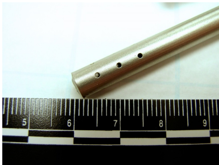
Figure 3.31. Photograph of small ports cut via waterjet into the aeration downtube.
