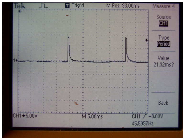
Figure 3.28. Photograph of oscilloscope measurements of the pulse-width modulation of LED light in experimental work.
