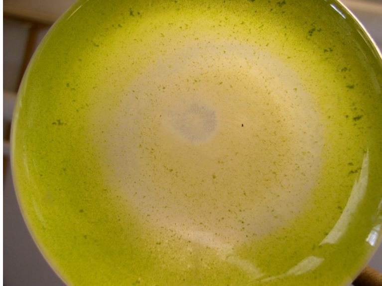
Figure 5.5. Example of biofilm formed in flashing (45.6 Hz) illumination under red (660 nm) light experiments.
