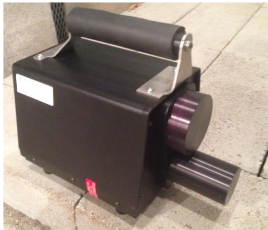
Fig. 1. N-Probe fast and thermal neutron spectrometer [9].
