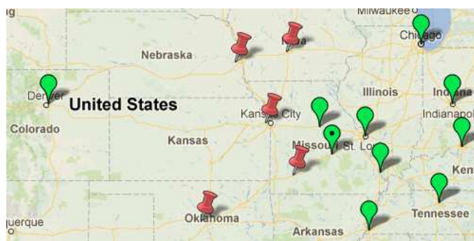
Figure 5: Result of clustering wind location: sites in the pin-shape correspond to the first cluster; sites in the balloon-shape correspond to the second cluster.
