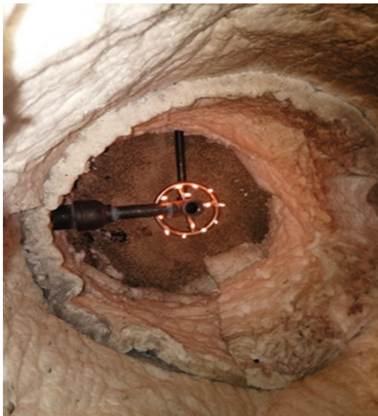
Figure 2.7. Top view of combustion chamber showing insulation, ring burner and syngas outlet opening
