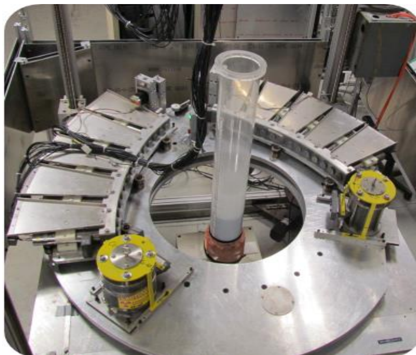
Figure 3. Photograph of the DSCT technique, and 0.152 m spouted bed inside the setup for scan.
