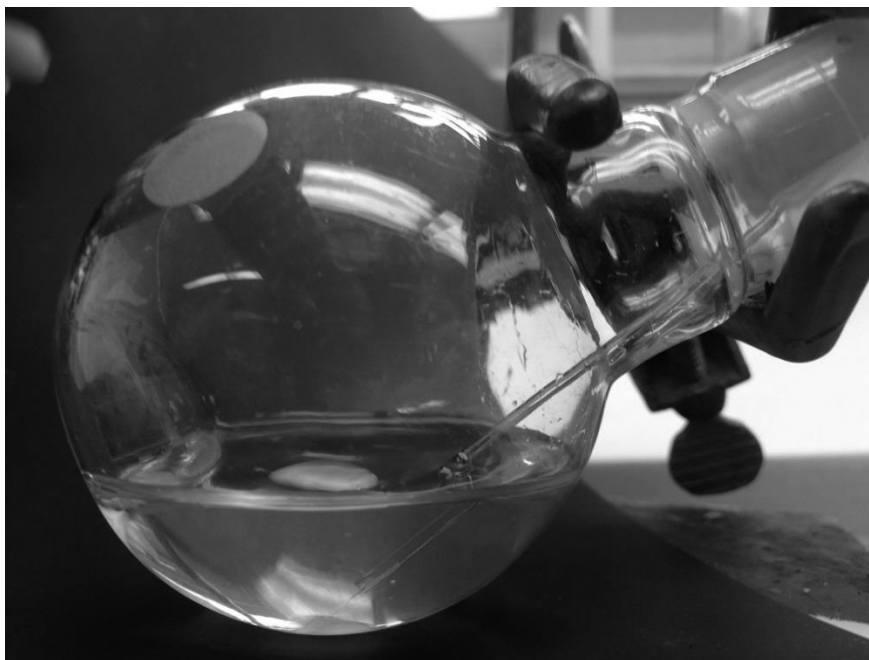
Fig. 17. Submerged water addition
