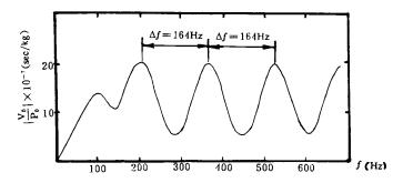
Fig. 2 Admittance Curve for Intact Pile
