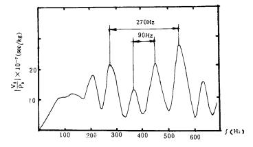
Fig. 4 Admittance Curve for Neck-Widened Pile
