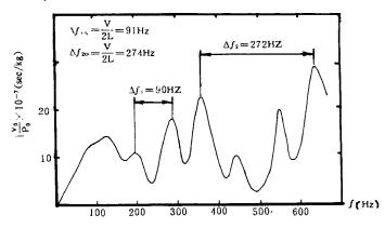
Fig. 3 Admittance Curve for Neck-Narrowed Pile
