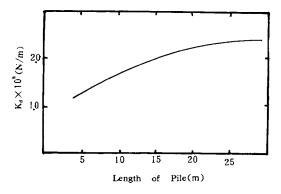
Fig. 5 Effects of Length of Pile on Stiffness
