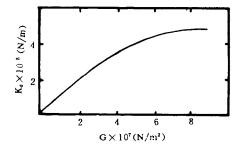
Fig . 6 Effects of  $E_s$  on stiffness as  $E_{\mbox{\tiny P}}$  keeping Constant
