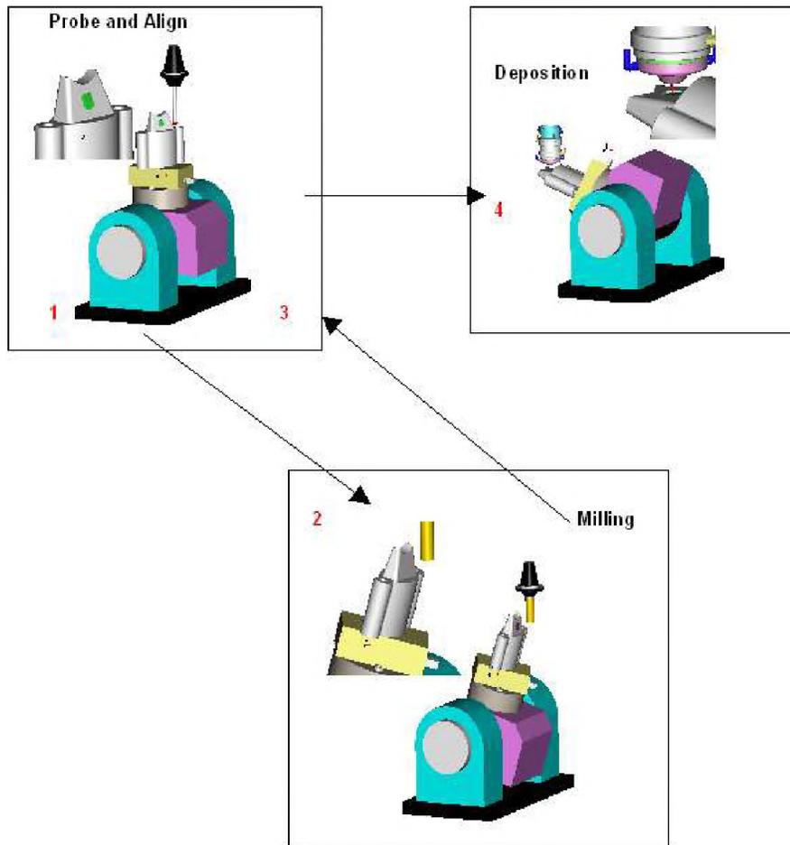
*Figure 1 – Repair Process*
