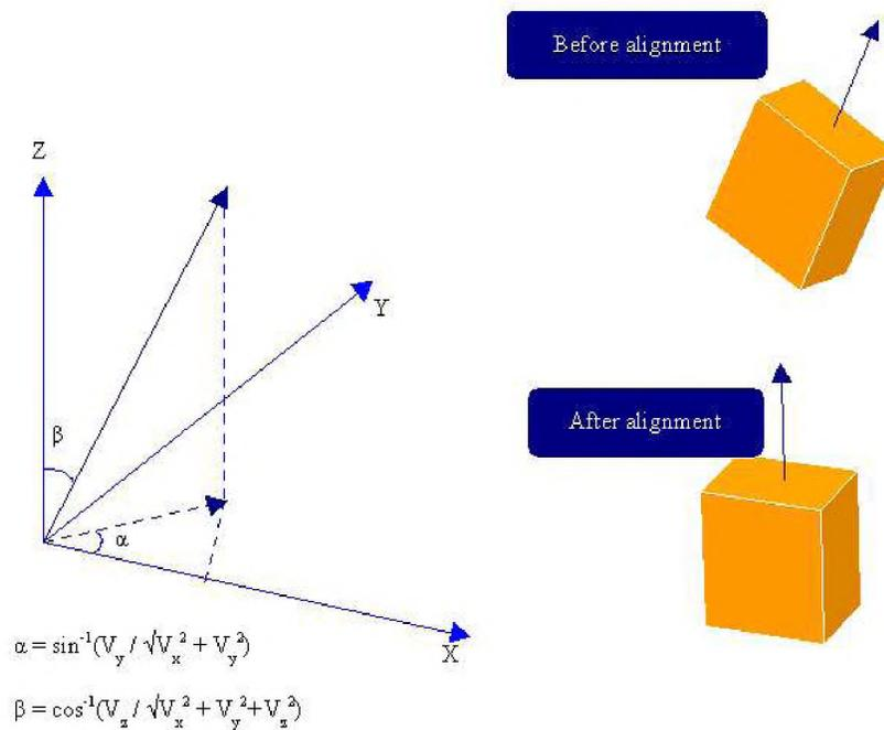
*Figure 3 – Surface Leveling*
