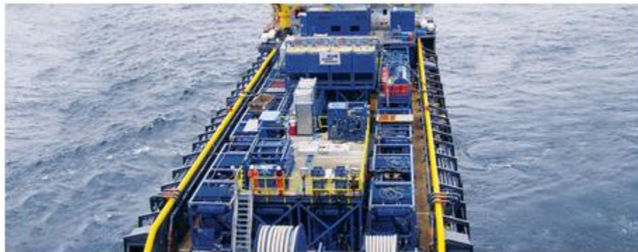
Figure 1.11. A view of the deck of a dynamically positioned stimulation vessel (DPSV) (Baker Hughes, 2013)
