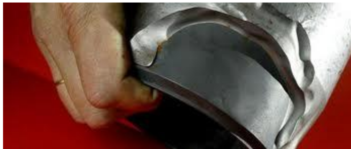
Figure 1.2. Erosion of downhole equipment due to sand production (Statoil, 2013)
