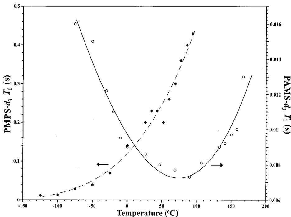
FIG. 5. The  $T_1$ 's from the typical three-parameter exponential fit for the  $\theta=90^\circ$  resonances of PAMS- $d_3$  ( $\circ$ ) and PMPS- $d_3$  ( $\blacklozenge$ ). The curves were drawn for clarity.
