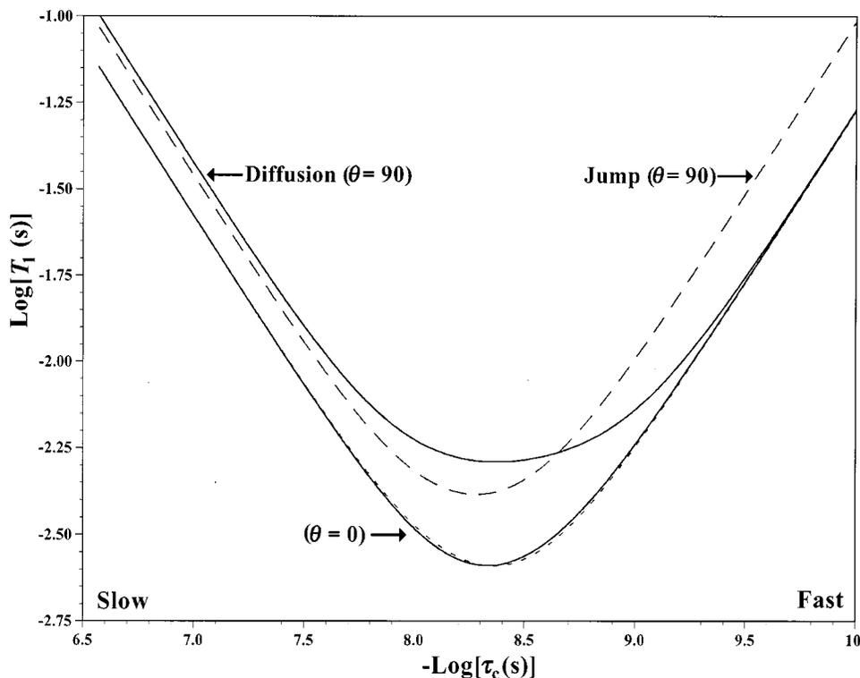
FIG. 1. Plots of the  $\theta=0^\circ$  and  $\theta=90^\circ$   $T_1$ 's as a function of  $\tau_c$  for the  $120^\circ$  jump (---) and diffusion (—) mechanisms.  $\tau_c=k^{-1}$  for jumps and  $D^{-1}$  for diffusion with  $k$  being the jump rate and  $D$  the diffusion constant.
