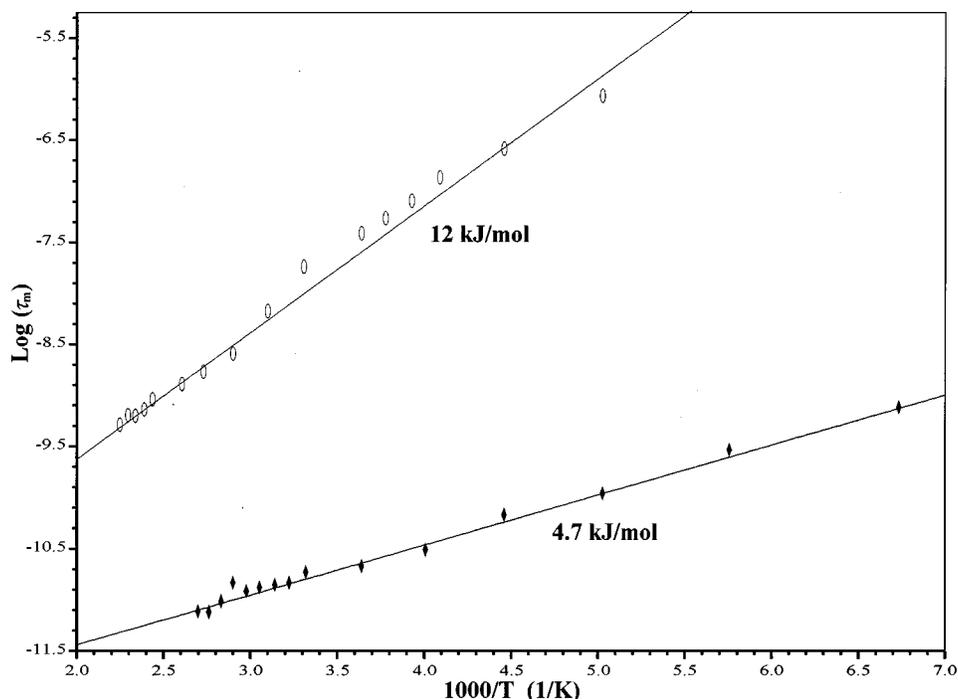
FIG. 9. The  $\tau_m$ 's or log-average  $\tau_c$ 's fit from the serial jump/diffusion model with a distribution of  $\tau_c$ 's as a function of inverse temperature for PAMS- $d_3$  ( $\circ$ ) and PMPS- $d_3$  ( $\blacklozenge$ ). The lines correspond to Arrhenius relations.
