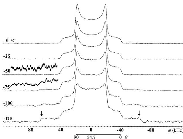
FIG. 2. Low-temperature solid-echo spectra of PAMS- $d_3$ . The  $\theta$  scale applies to the transition that has its horn or maxima around 19 kHz. The arrows on the  $-120^\circ\text{C}$  spectrum mark the horns of the "frozen" methyl powder pattern which is only evident at  $-50$  and  $-75^\circ\text{C}$  as an increased baseline.
