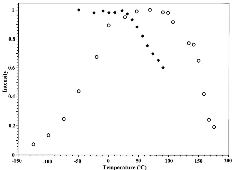
FIG. 4. Boltzmann corrected spectral intensities for PAMS- $d_3$  ( $\circ$ ) and PMPS- $d_3$  ( $\blacklozenge$ ). The decrease above 100 °C for PAMS- $d_3$  and the decrease for PMPS- $d_3$  are from backbone motion. The low-temperature decrease of PAMS- $d_3$  is from intermediate region methyl rotation.
