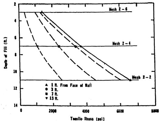
Figure 4. Tensile Stress in Reinforcing Mesh (Site 2)
