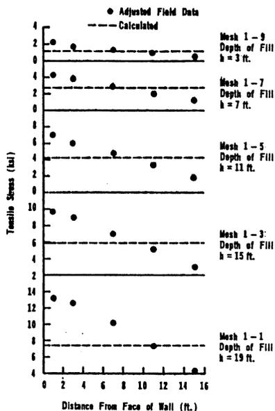
Figure 5. Tensile Stress Distribution Along Reinforcing Mesh (Site 1)
