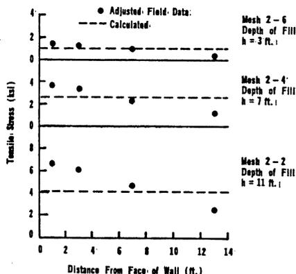
Figure 6. Tensile Stress Distribution Along Reinforcing Mesh (Site 2)
