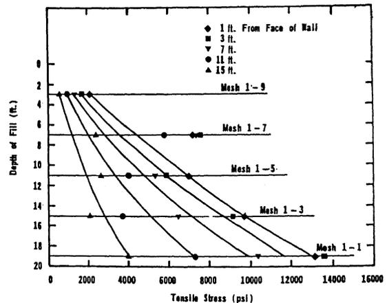
Figure 3. Tensile Stress in Reinforcing Mesh (Site 1)
