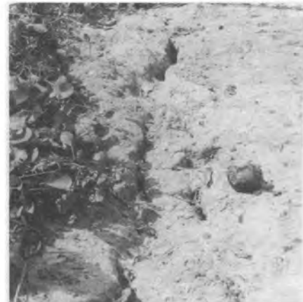
Fig. 8. Fissure housing sand boils in loose sand, near high tide level during Great Nicobar earthquake.
