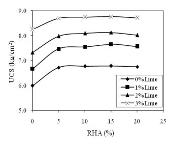
Fig. 4. Curing Effect on unconfined compressive strength of RHA mixed alluvial soil with varying percentage of Lime
