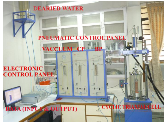
Fig. 3. Cyclic triaxial equipment set-up
