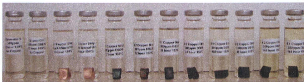
Figure 1.18. Copper strips exposed to white mineral oil fortified with DBDS
