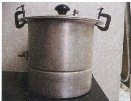
Figure 8.1. Aluminum desiccator with two bulkhead fittings with gas tight septum
