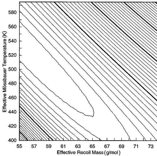
FIG. 6. A contour plot of the values of the effective recoil mass and the effective Debye or Mössbauer temperature which are consistent with the isomer shifts observed in  $\text{Ce}_{0.98}\text{Fe}_4\text{Sb}_{12}$ . Any pair of values found within the inner contour will fit the experimental isomer shifts within the experimental errors. Each major and minor contour corresponds, respectively, to a 0.0005 and a 0.00005 increase in the sum of squares misfit.
