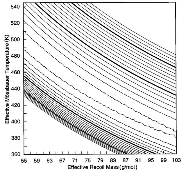
FIG. 8. A contour plot of the values of the effective recoil mass and the effective Mössbauer temperature which are consistent with the Mössbauer spectral absorption areas observed in  $\text{Ce}_{0.98}\text{Fe}_4\text{Sb}_{12}$ . Any pair of values found within the inner contour will fit the experimental values within the experimental errors. Each major and minor contour corresponds, respectively, to a 0.001 and a 0.00015 increase in the sum of squares misfit.
