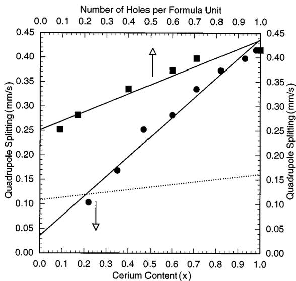
FIG. 2. The variation with Ce content  $x$ , ●, and with the number of holes per formula unit, ■, of the 295-K quadrupole splitting observed in Ce<sub>x</sub>Fe<sub>4-y</sub>Co<sub>y</sub>Sb<sub>12</sub>. The dashed line represents a point-charge calculation of the lattice contribution to the quadrupole splitting as is discussed in the text. The error bars are essentially the size of the data points.
