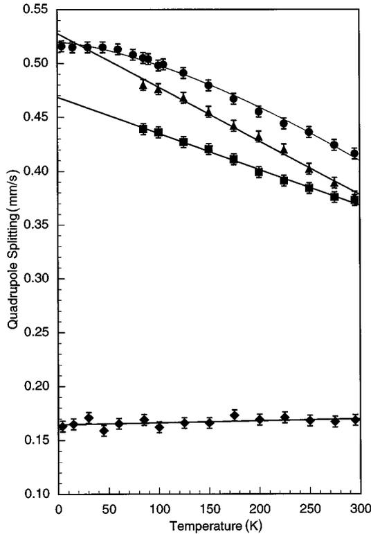
FIG. 3. The temperature dependence of the quadrupole splittings observed in  $\text{Ce}_{0.35}\text{FeCo}_3\text{Sb}_{12}$ ,  $\blacklozenge$ ,  $\text{Ce}_{0.60}\text{Fe}_2\text{Co}_2\text{Sb}_{12}$ ,  $\blacktriangle$ ,  $\text{Ce}_{0.82}\text{Fe}_3\text{CoSb}_{12}$ ,  $\blacksquare$ , and  $\text{Ce}_{0.98}\text{Fe}_4\text{Sb}_{12}$ ,  $\bullet$ . The  $\text{Ce}_{0.98}\text{Fe}_4\text{Sb}_{12}$  results have been fit with Eq. (3), see text.
