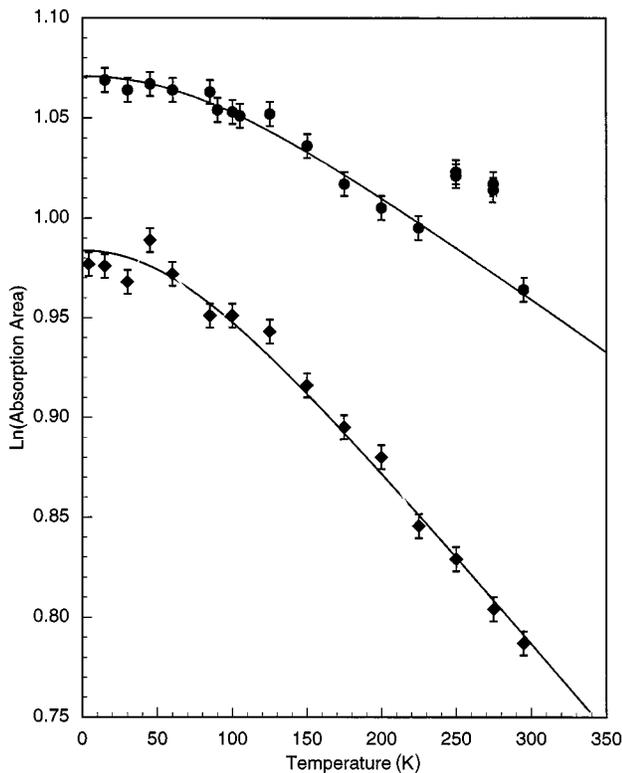
FIG. 7. The temperature dependence of the logarithm of the Mössbauer spectral absorption areas observed for  $\text{Ce}_{0.35}\text{FeCo}_3\text{Sb}_{12}$ ,  $\blacklozenge$ , and  $\text{Ce}_{0.98}\text{Fe}_4\text{Sb}_{12}$ ,  $\bullet$ .
