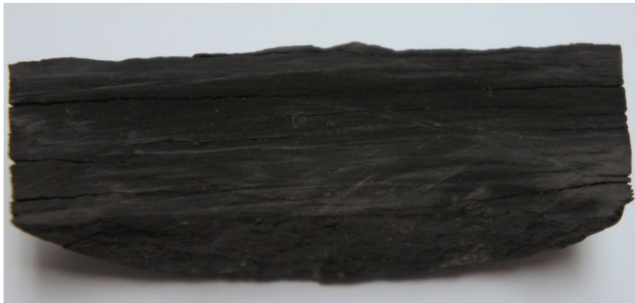
Figure 3.3. Bulk shale cracked when fluid is introduced
