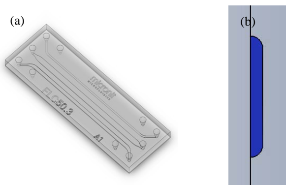
Figure 4.10. Microfluidic chip with microfractures (a) and cross-sectional view of a single fracture (b)
