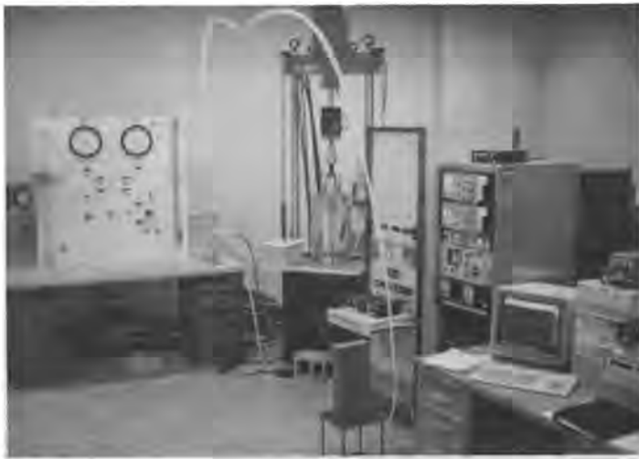
Figure 1. Experimental System for Hollow Cylinder Testing
