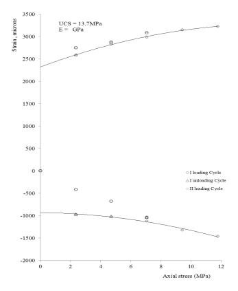
Fig.3. Strain v/s Stress (Ujh-2sample)
