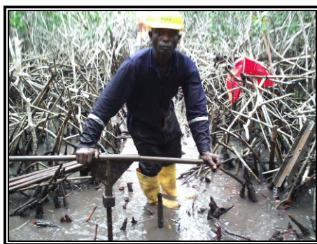
Fig. 9: The Cone Penetrometer Test being carried out along the Andoni River to Bonny River East-West Coastal Road Alignment.
