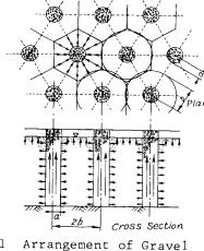
Fig.l Arrangement of Grave Drain System
