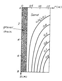
Fig.3 Variation of Pore Water Pressure Ratio with Space
