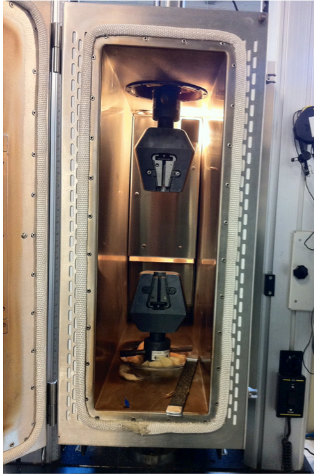
Figure 5.7 The strain frame encased inside the furnace for simultaneous application of temperature and strain.
