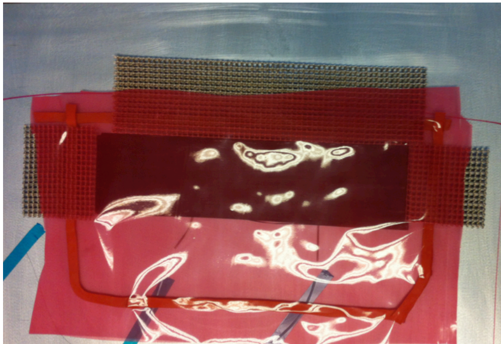
Figure A.1 BMI sample assembly with the optical fiber sensor before cure process.
