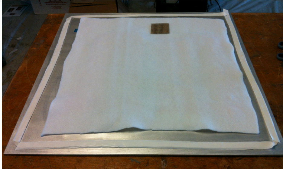
Figure A.3 Sample assembly covered with the breather fabric.
