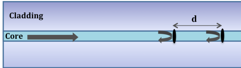
Figure 3.2 Schematic of an IFPI sensor consisting of two reflecting surfaces on the fiber core.
