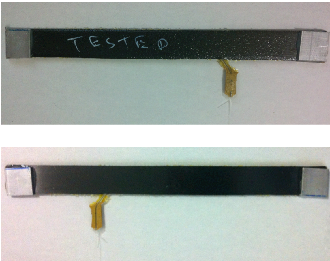
Figure A.7 Prepared BMI sample with aluminum tabs attached.
