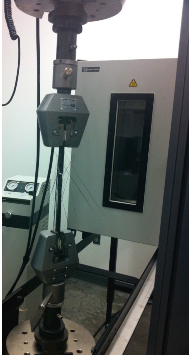
Figure B.3 Complete sample failure due to large exerted strain.
