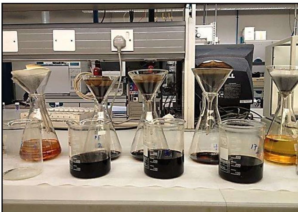
Figure 3.18. Apparatus for Filtering Dirt out of Oil
