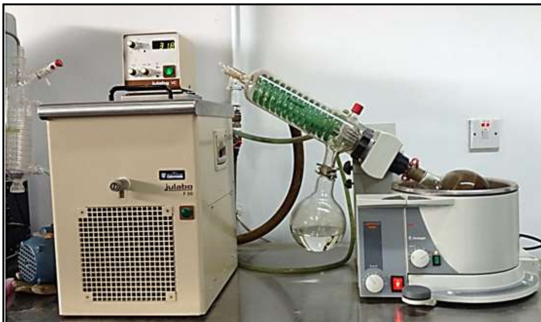
Figure 3.19. Apparatus for Separating Oil from Extraction Fluids
