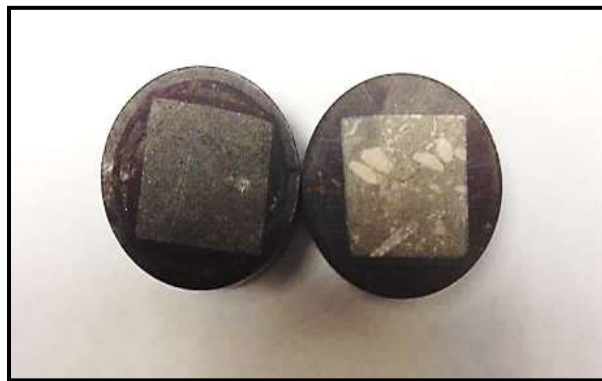
Figure 3.7. Cuboid-Shaped Samples Coated with Viscous Epoxy in a 1 in ID Acrylic Tube
