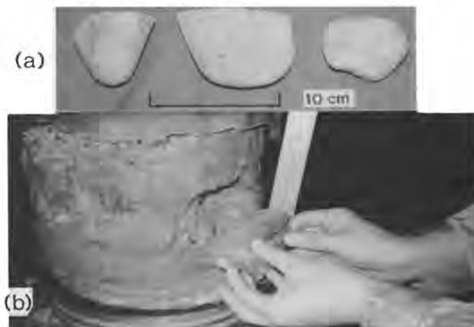
Fig. 8 (a) Gravels cut during core boring and (b) view of a specimen after test (A piece of gravel being removed from the specimen)
