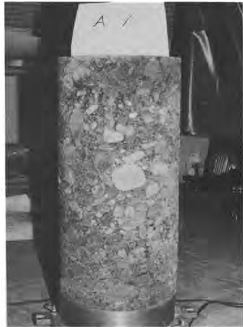
Fig. 3.5 Undisturbed frozen gravel sample (30cm in diameter, 60 cm high)
