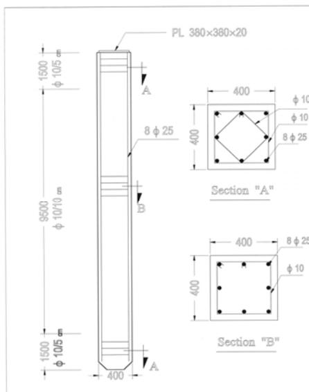
Fig. 1. Details of precast test uniform pile
