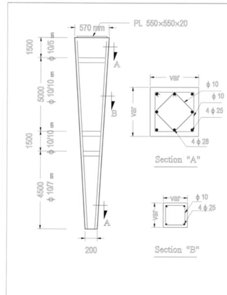
Fig. 2. Details of precast test tapered pile
