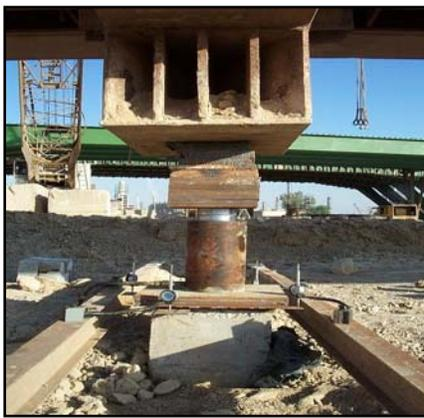
Fig. 4. Static loading test on pile
