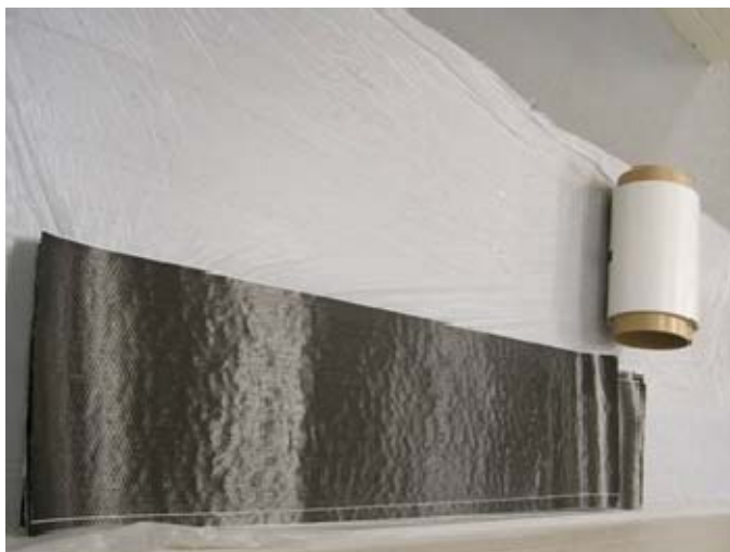
(a) Unidirectional carbon fiber sheet
