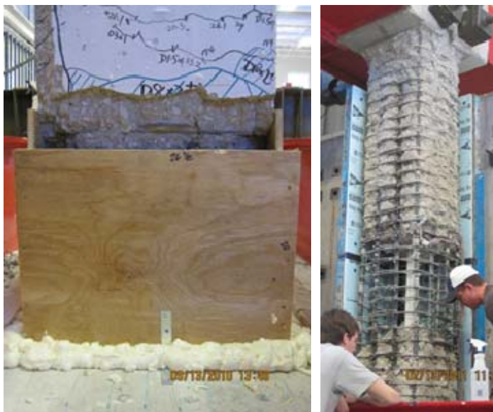
(a) Plywood Formwork
