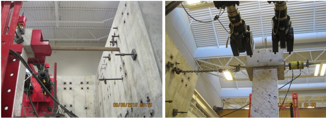
Figure A.1. Column Straightening
