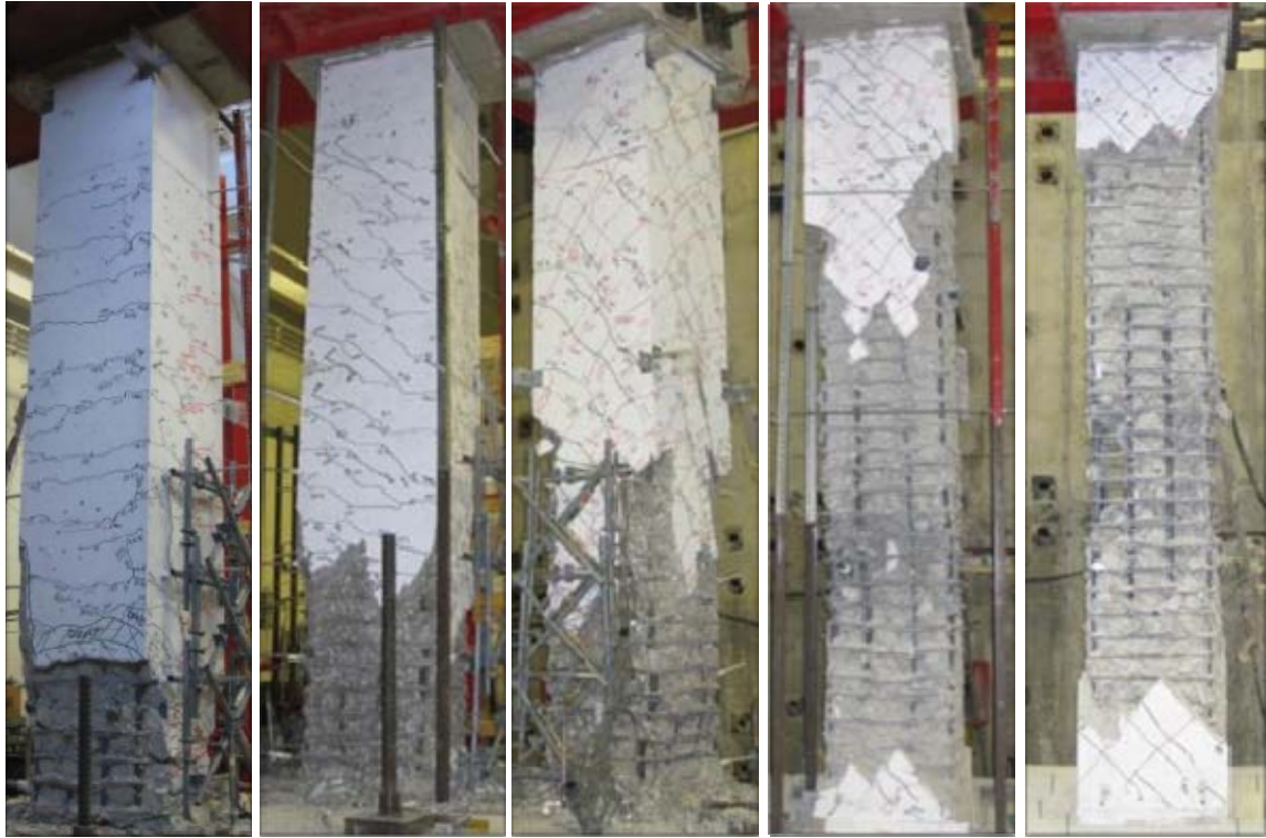
Column 1 (T/M=0) Column 2 (T/M=0.2) Column 3 (T/M=0.4) Column 4 (T/M=0.6) Column 5 (T/M=∞)
